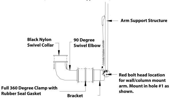
This is the new location for the red bolt. This is how the joint should look when it is ready to be mounted.
