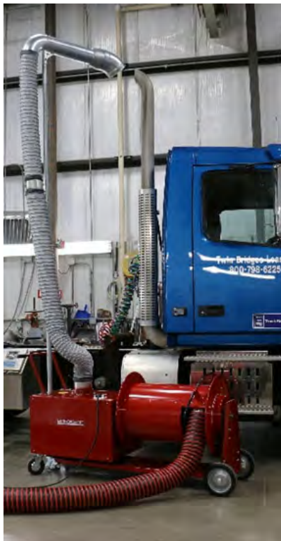
Eliminator Hose Reel Model connected to truck using extended vertical mast
