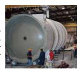
sel and the duct. Corrosion resistant fiberglass duct and process vessels have proven to be the best choice. The net result is a sound financial and environmental solution.
